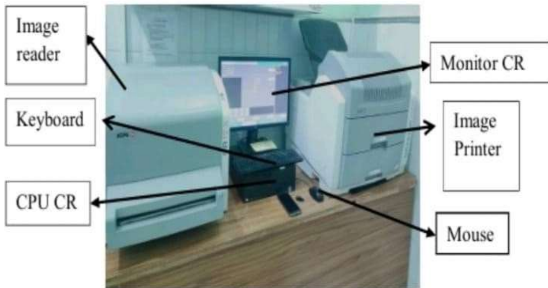
Figure 3. Computer Radiography, Image Reader and Image Printer at Haji General Hospital, Medan
