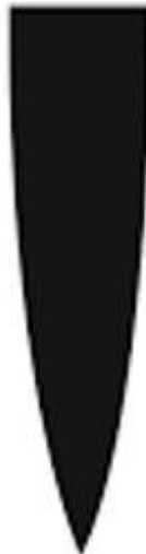
Figure 5. Standard Knife Blade Shape for the Animal Slaughter Industry (Convex Shape)
